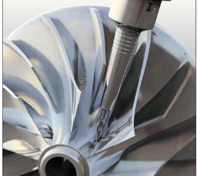
5축 볼엔드밀 정삭가공 Finishing with ball endmill on 5-axis machine
